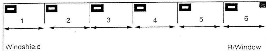
To measure for the headliner, start at the front windshield on center, measure from windshield to front/face side of bow #1, #1 to face side #2, etc. To top side of rear window.
